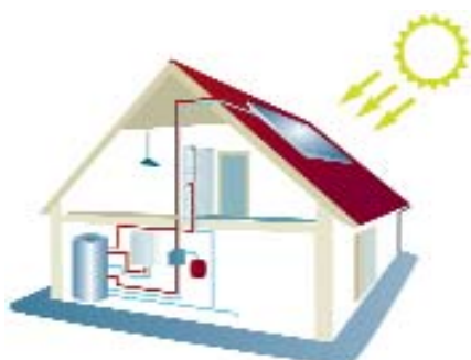
figure 35: flat panel solar technology
